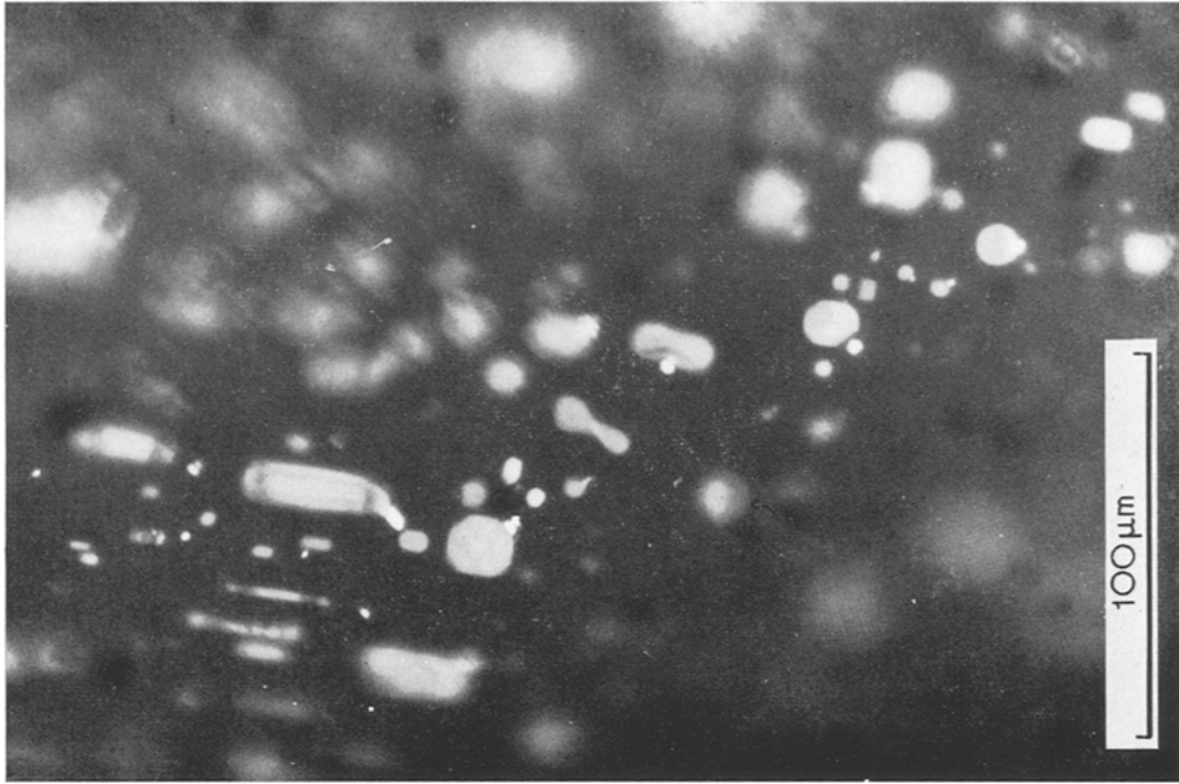
Figure 2 Voids on a subgrain boundary. The voids are in focus only in the central region of the sloping boundary. The white specks close to the voids are bright gold precipitates.
