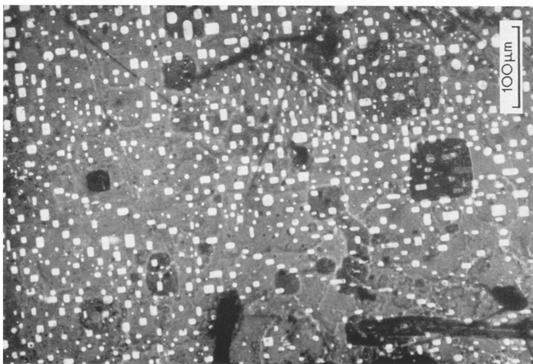
Figure 3 Planar array of voids 10 μm below the surface. The sloping line on the left hand corner is the trace of a subgrain boundary.
